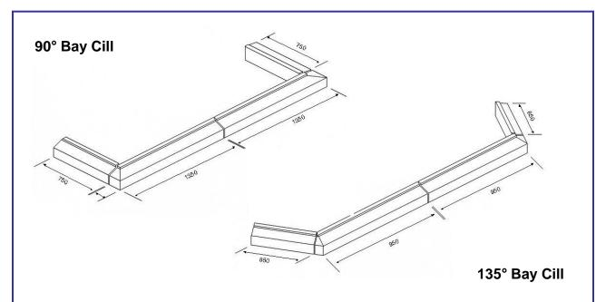
Bay window sets can be cut to suit brickwork size required, alternatively the cills can be manufactured to the customers brickwork dimensions in any of the sections shown on the opposite page.
